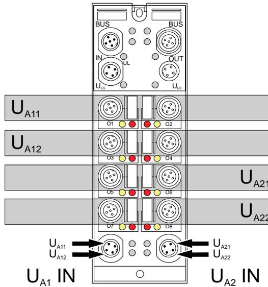
Fig. 6-32 Output supply (digital output device, e.g., RF-FLS IB M12 DO 8 M12-2A)
