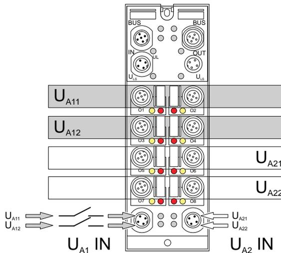
Fig. 6-39 Switching off specific outputs (RF-FLS)
