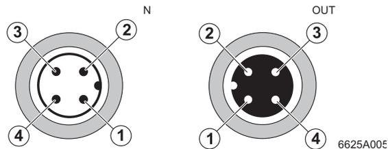
Fig. 6-14 Pin assignment of the power supply  $U_{LS}$  (connections on the Fieldline Stand-Alone device)
