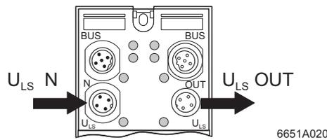
Fig. 6-13 Connections for the power supply  $U_{LS}$  (RF-FLS)
