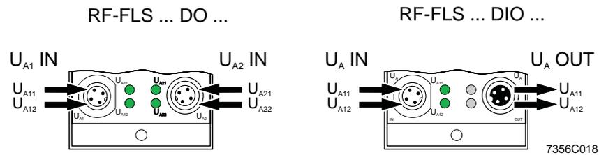
Fig. 6-23  $U_A$  connections for DO and DIO devices (RF-FLs M12)
