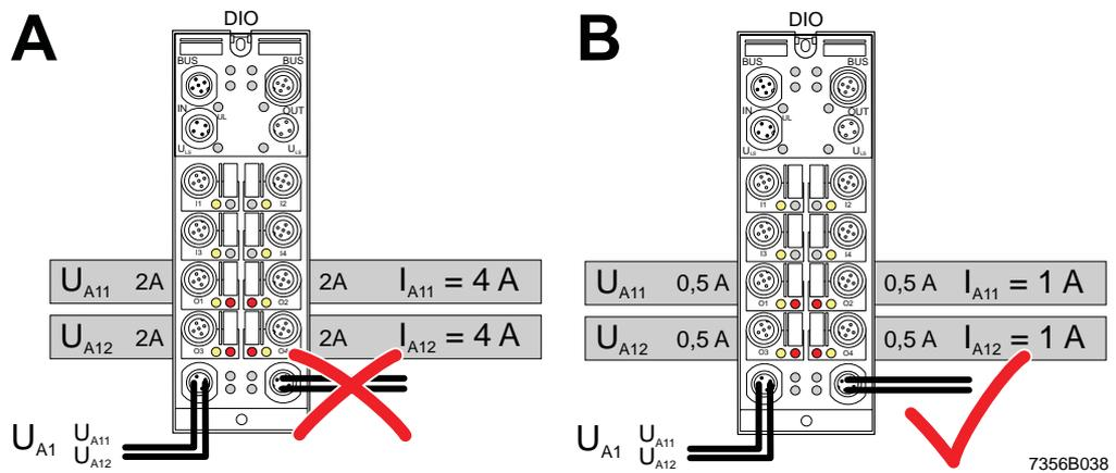
Fig. 6-47 Forwarding the supply voltage
