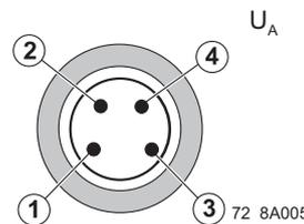
Fig. 6-29 Pin assignment of the power supply  $U_A$  of the outputs (connections on the Fieldline Modular M8 device)
