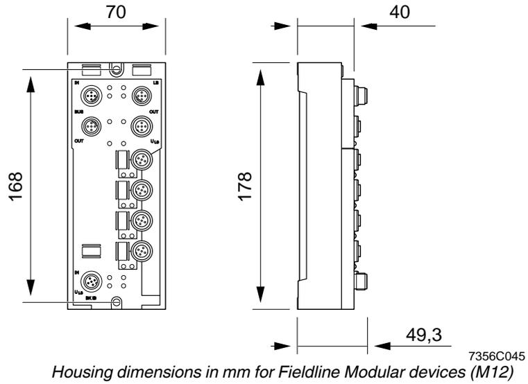
Fig. 5-2 Housing dimensions in mm for Fieldline Modular devices (M12)
