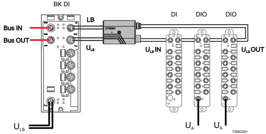
Fig. 6-37 Example for the supply and forwarding of supply voltages (RF-FLM M8)
