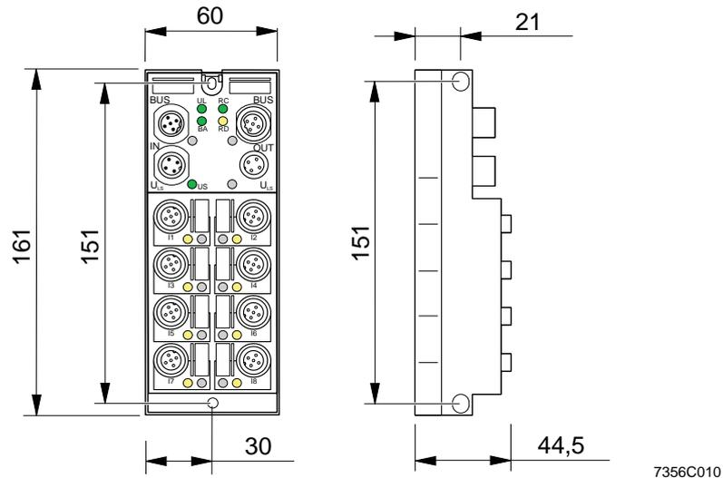
Fig. 4-2 Housing dimensions in mm for Fieldline Stand-Alone devices without actuator supply
