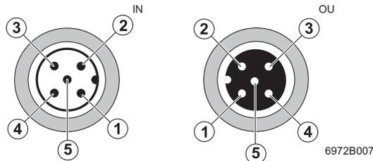
Fig. 6-27 Pin assignment of the power supply  $U_A$  of the outputs (connections on the Fieldline Modular device)
