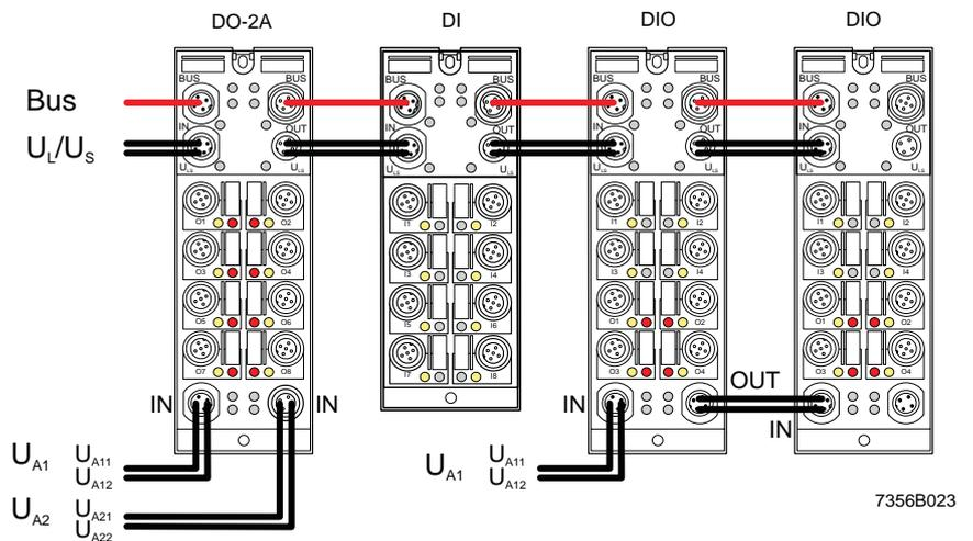
Fig. 6-36 Example for the supply and forwarding of supply voltages (FLS)
