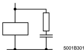
Fig. 6-2 Relay coil with RC element
