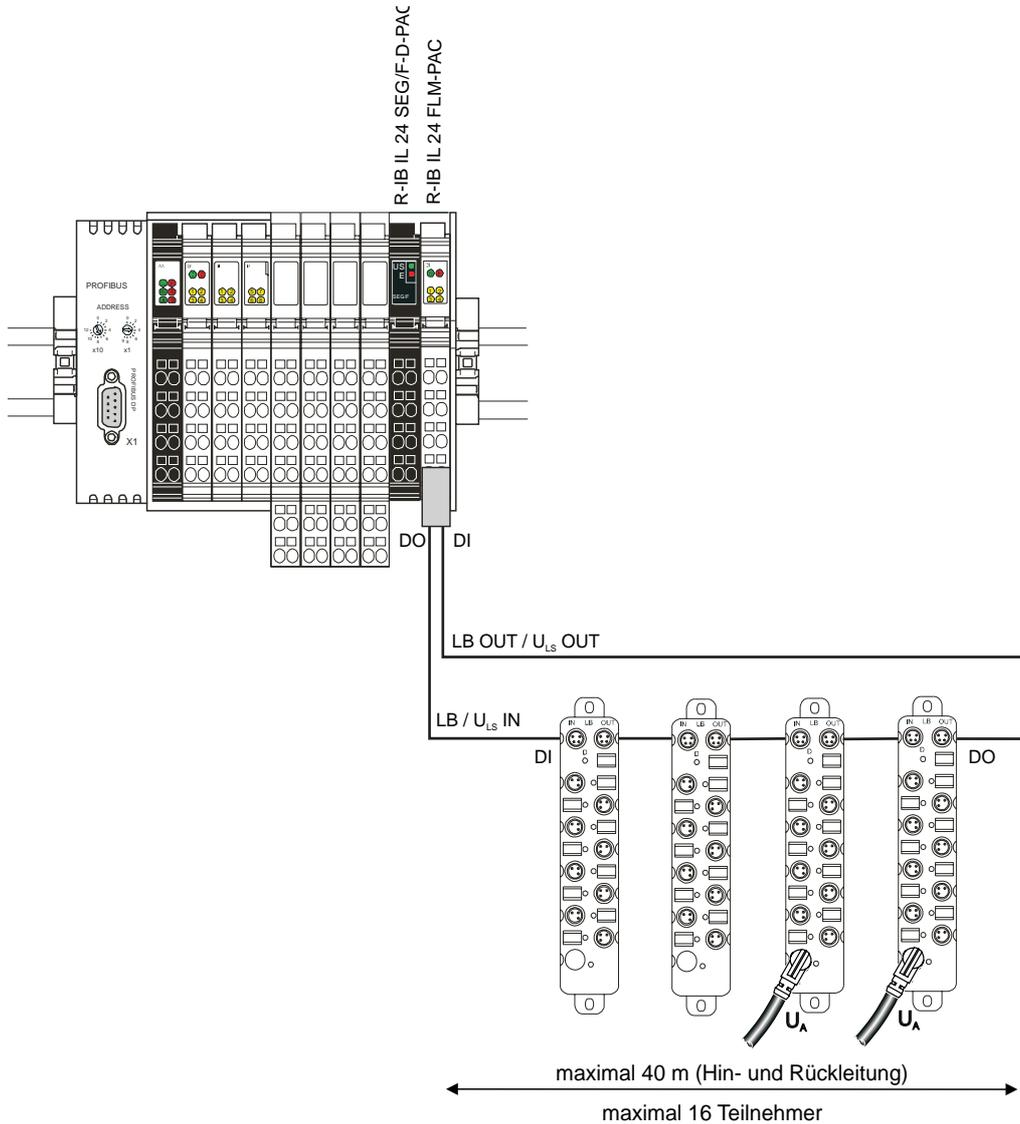
Fig. 5-9 Typical structure of a Fieldline Modular M8 station at Inline 7356C072
