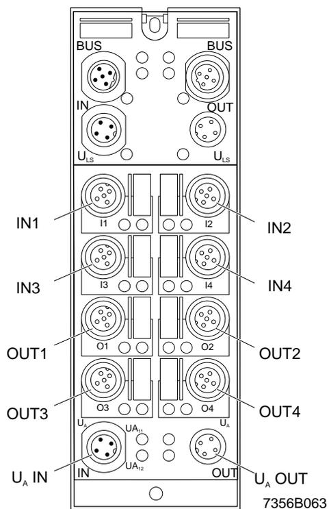
Fig. 6-41 RF-FLS M12 DIO 4/4 M12-2A
