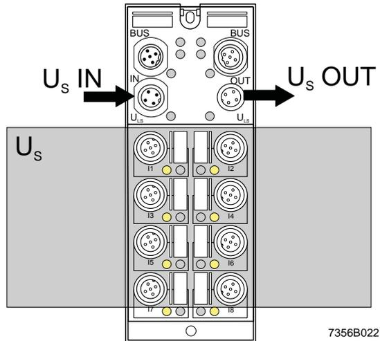
Fig. 6-31 Input supply (digital input device, e.g., RF-FLS IB M12 DI 8 M12)
