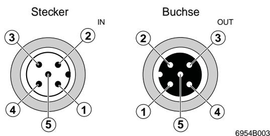
Fig. 6-18 Pin assignment of the power supply  $U_{LS}$  (connections on the Fieldline Modular M12 device)
