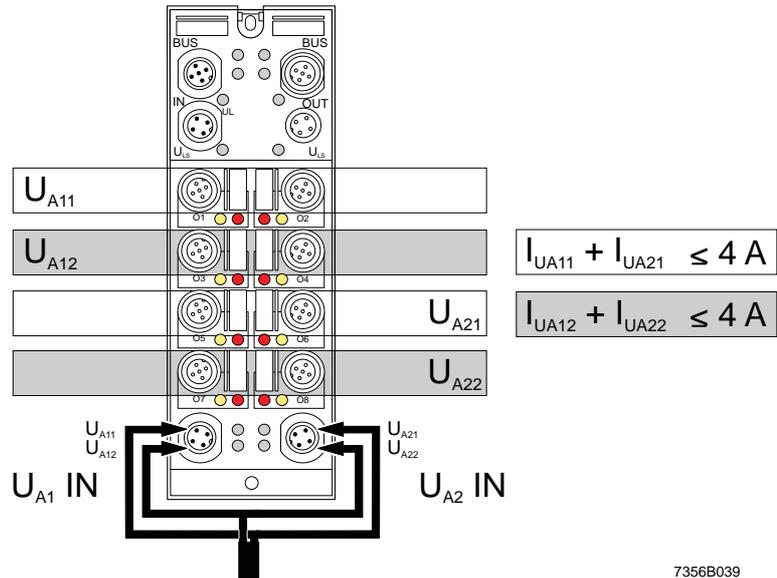
Fig. 6-38 Supply via a Y cable (RF-FLS)
