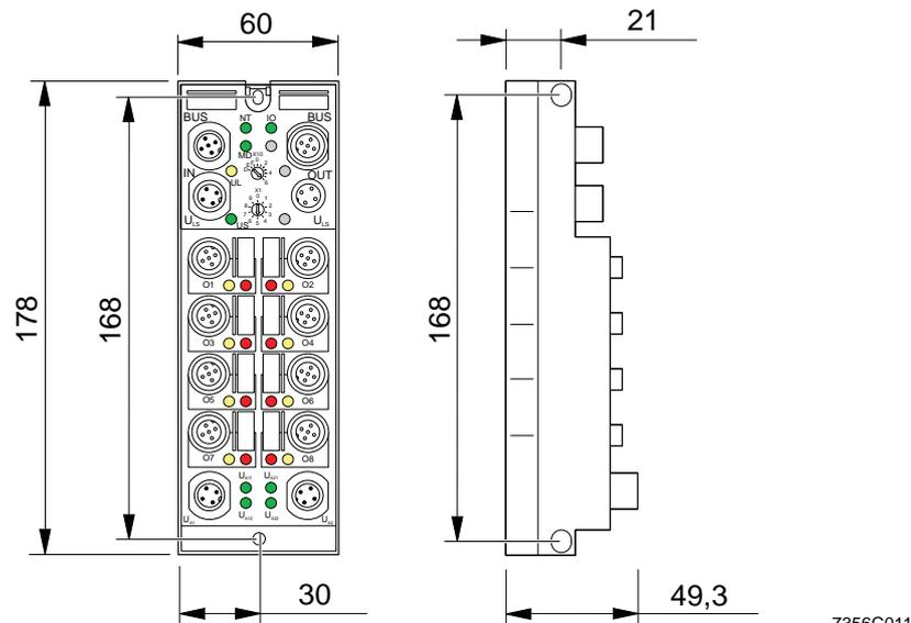
Fig. 4-3 Housing dimensions in mm for Fieldline Stand-Alone devices with actuator supply
