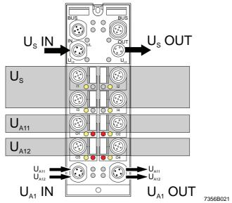
Fig. 6-33 Input and output supply (digital I/O device, e.g., RF-FLS IB M12 DIO 4/4 M12-2A)
