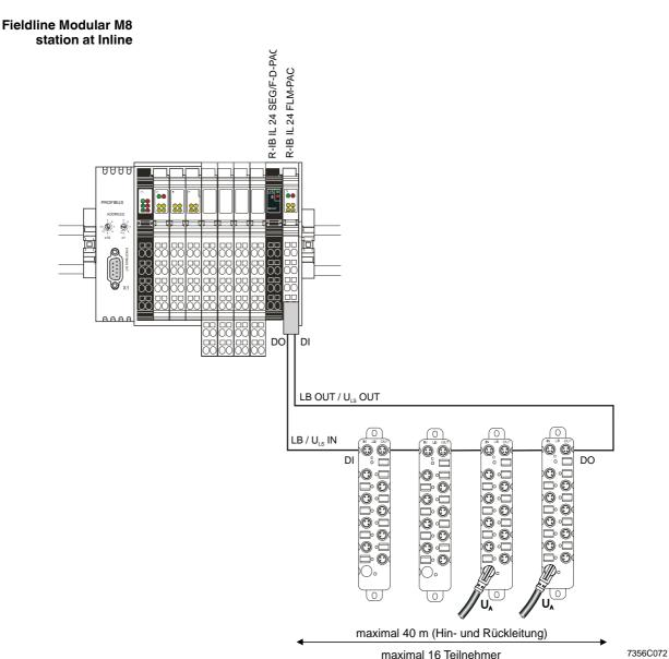
Fig. 5-9 Typical structure of a Fieldline Modular M8 station at Inline
