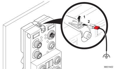
Fig. 6-5 Functional earth grounding via external FE connection for front mounting (FLS)
