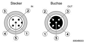
Fig. 6-18 Pin assignment of the power supply U<sub>LS</sub> (connections on the Fieldline Modular M12 device)
