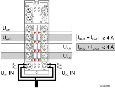
Fig. 6-38 Supply via a Y cable (RF-FLS)
