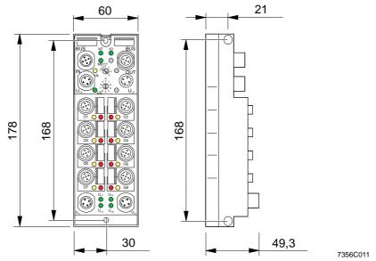
Fig. 4-3 Housing dimensions in mm for Fieldline Stand-Alone devices with actuator supply
