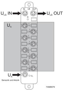
Fig. 6-35 Input and output supply (digital I/O device, e.g., RF-FLM DIO 8/4 M8)
