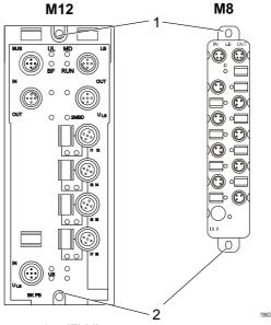
Fig. 6-8 Front mounting (FLM)
