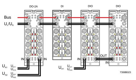
Fig. 6-36 Example for the supply and forwarding of supply voltages (FLS)
