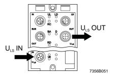
Fig. 6-16 Connections for the power supply  $U_{LS}$  on the bus coupler (RF-FLM)
