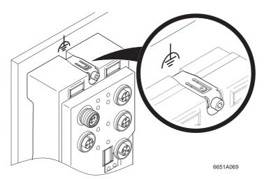
Fig. 6-9 Functional earth grounding with grounded mounting surface (RF-FLM M12)
