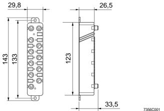
Fig. 5-3 Housing dimensions in mm for Fieldline Modular devices (M8)
