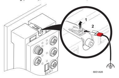
Fig. 6-10 Functional earth grounding via external FE connection (RF-FLM M12)
