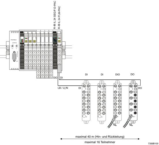
Fig. 6-46 Fieldline Modular M8 station connected to Inline
