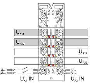
Fig. 6-39 Switching off specific outputs (RF-FLS)
