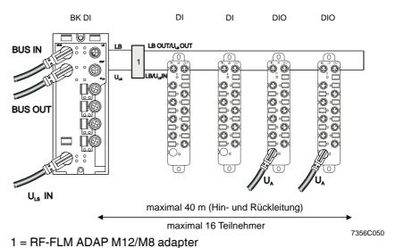
Fig. 5-8 Example structure of a Fieldline Modular M8 station
