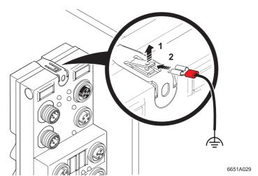
Fig. 6-7 Functional earth grounding via external FE connection for side mounting (FLS)
