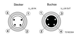
Fig. 6-21 Pin assignment of the power supply  $U_{LS}$  and the local bus (RF-FLM M8)
