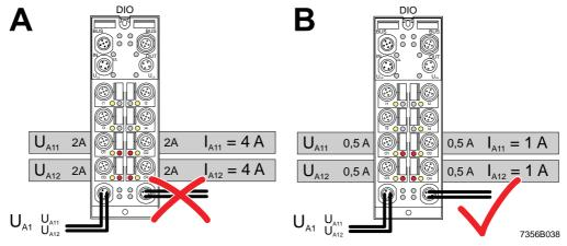
Fig. 6-47 Forwarding the supply voltage
