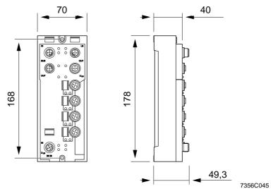
Fig. 5-2 Housing dimensions in mm for Fieldline Modular devices (M12)
