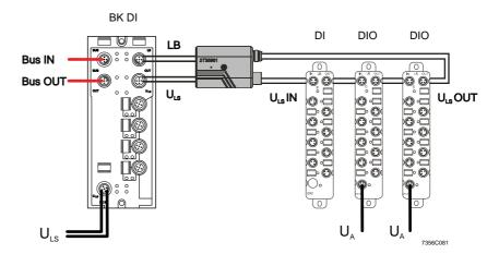
Fig. 6-37 Example for the supply and forwarding of supply voltages (RF-FLM M8)
