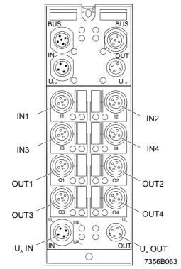
Fig. 6-41 RF-FLS M12 DIO 4/4 M12-2A
