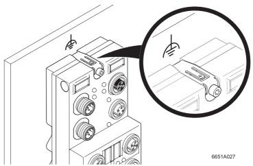
Fig. 6-4 Functional earth ground connection for a grounded mounting surface (FLS)
