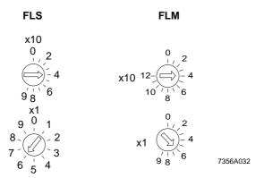
Fig. 6-12 Example: Address 46 (RF-FLS and RF-FLM)
