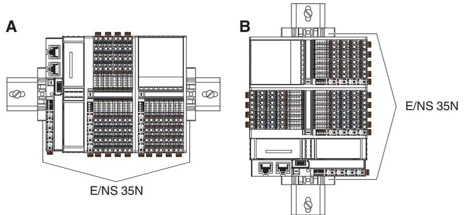
Fig. 6-3 Mounting positions for an IndraControl S20 station
