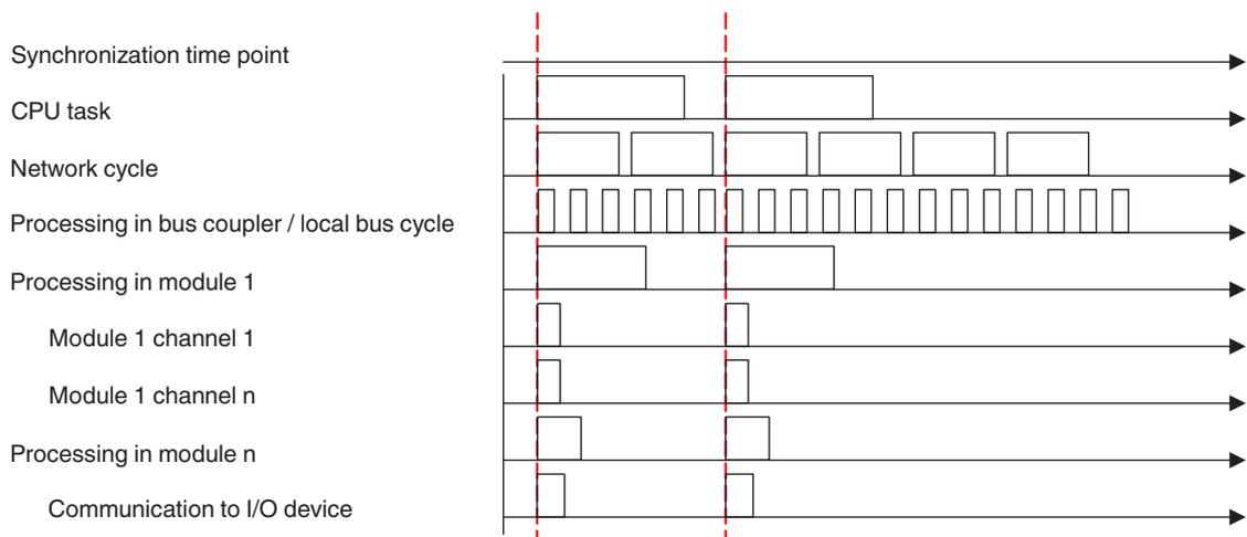
Fig. 13-14 Synchronous
