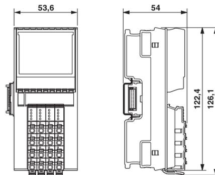
Fig. 5-15 Nominal dimensions of the F housing for the low voltage area with one terminal field and four connectors (type 1F-LV4: e.g., S20-DOR-4/2-220-AC)
