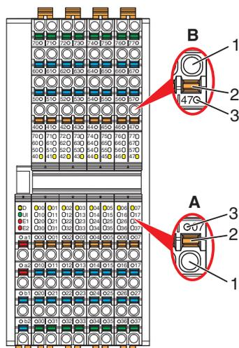
Fig. 7-4 Terminal point with associated spring lever, and associated touch connection
