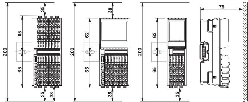
Fig. 6-19 Mounting distances: I/O modules (dimensions rounded)
