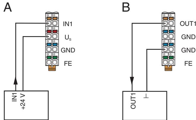
Fig. 7-16 2-wire connection for digital modules
