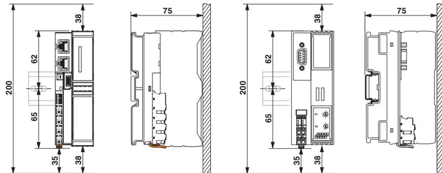
Fig. 6-18 Mounting distances: bus coupler (dimensions rounded)
