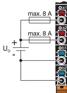
Fig. 7-12 Parallel supply of the supply voltage
