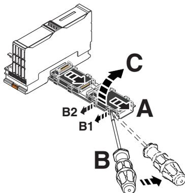
Fig. 6-13 Removing the bus base module
