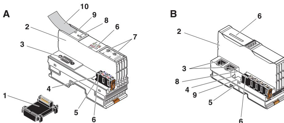
Fig. 5-4 Design of a bus coupler
