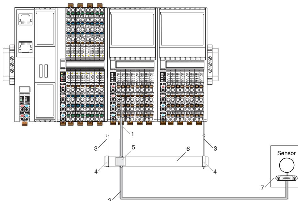
Fig. 8-2 Connecting the shield with the S20-SHIELD-SET
