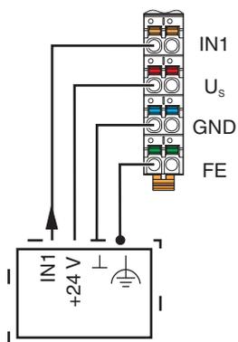
Fig. 7-18 4-wire connection for digital modules
