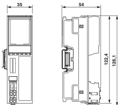
Fig. 5-14 Nominal dimensions of the H housing with one terminal field and short connectors
