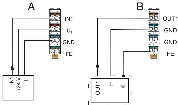
Fig. 7-17 3-wire connection for digital modules
