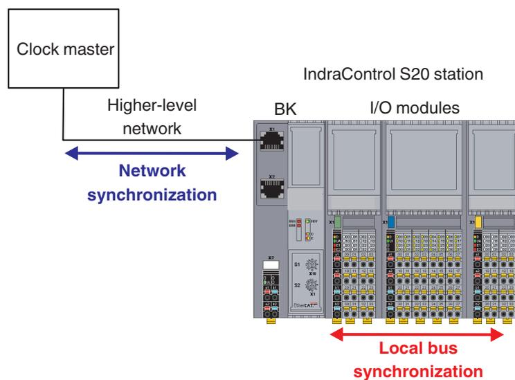
Fig. 13-11 Network and local bus synchronization
