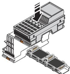
Fig. 6-10 Mounting input/output modules
