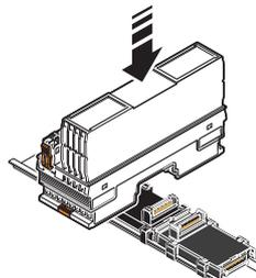
Fig. 6-7 Snapping the bus coupler on
