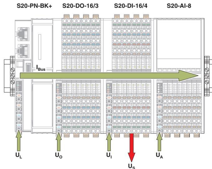
Fig. 7-10 Supply voltages in the IndraControl S20 system
