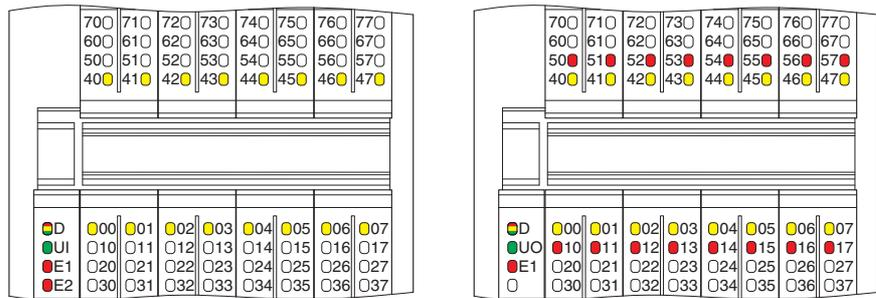
Fig. 9-5 LEDs on the I/O connectors (e.g., S20-DI-16/4, S20-DO-16/3)
