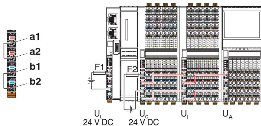
Fig. 7-11 Jumpering in the power connector and example of potential forwarding
