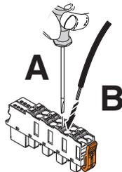
Fig. 7-6 Connecting a stranded cable
