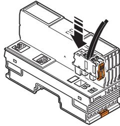
Fig. 7-7 Inserting the connector
