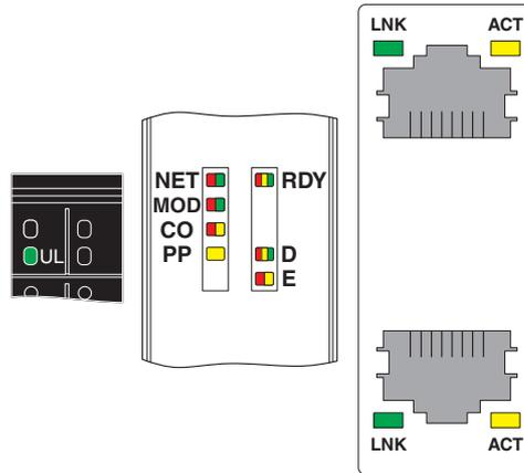
Fig. 9-1 Indicators on bus couplers (example: S20-EIP-BK)
