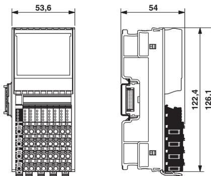
Fig. 5-10 Nominal dimensions of the F housing with one terminal field (type 1F: e.g., S20-AI-8, S20-DI-32/1)
