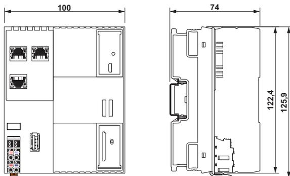
Fig. 5-6 Nominal dimensions of the controller housing (type XM2x: e.g., XM21)
