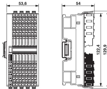
Fig. 5-9 Nominal dimensions of the F housing with two terminal fields (type 2F: e.g., S20-DI-16/4, S20-DO-16/3)
