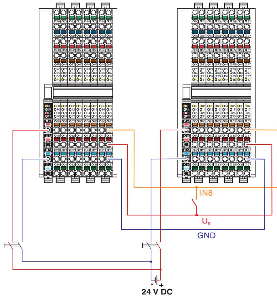
Fig. 7-19 Example: connection for redundant use
