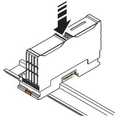
Fig. 6-8 Snapping the bus coupler on
