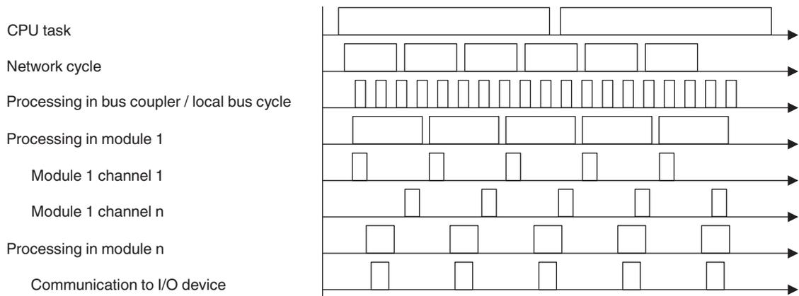
Fig. 13-13 Asynchronous
