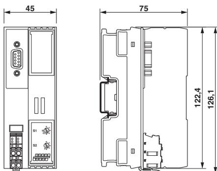
Fig. 5-7 Nominal dimensions of the bus coupler housing with separate bus base (type BK+: e.g., S20-PB-BK, S20-PN-BK+)
