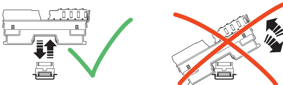
Fig. 6-1 *Placing/removing the module vertically*
