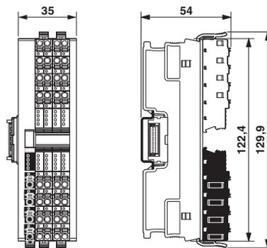
Fig. 5-11 Nominal dimensions of the H housing with two terminal fields (type 2H)
