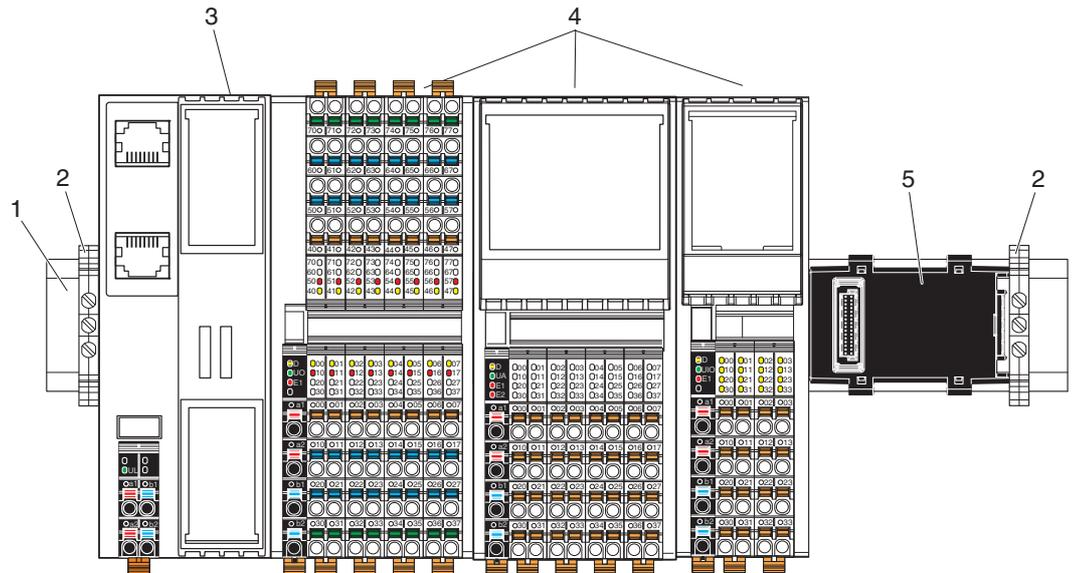
Fig. 3-1 Example of an IndraControl S20 station
