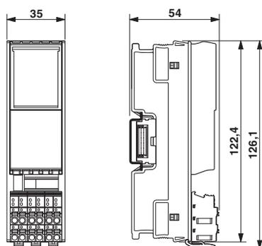
Fig. 5-13 Nominal dimensions of the H housing with one terminal field and short connectors
