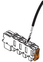
Fig. 7-5 Connecting a solid unshielded cable
