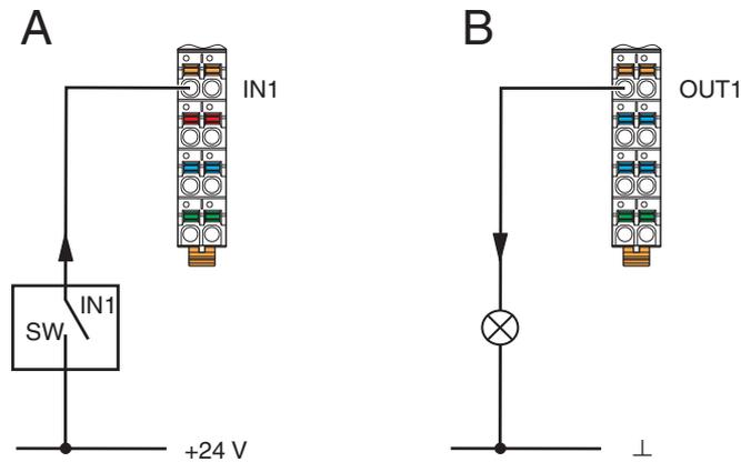
Fig. 7-15 1-wire connection for digital modules
