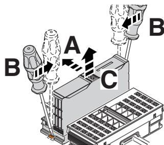
Fig. 6-14 Removing the bus coupler
