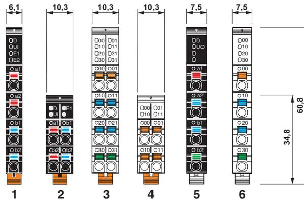
Fig. 5-19 Connectors: versions and dimensions
