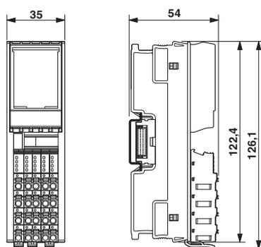
Fig. 5-12 Nominal dimensions of the H housing with one terminal field
