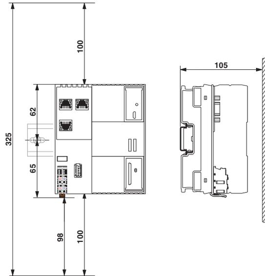
Fig. 6-17 Mounting distances: XM2x controller (dimensions rounded)
