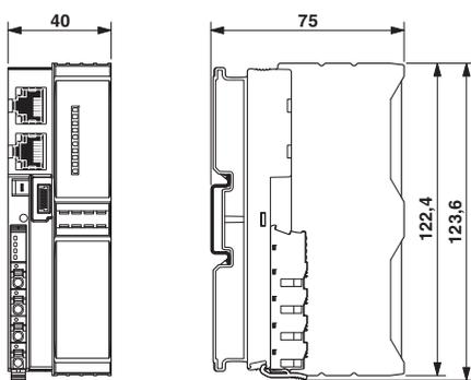
Fig. 5-8 Nominal dimensions of the bus coupler housing with integrated bus base (type BK: e.g., S20-PN-BK)
