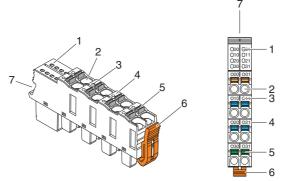
Fig. 5-21 Basic design of an IndraControl S20 connector
