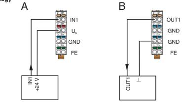
Fig. 7-16 2-wire connection for digital modules
