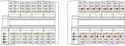
Fig. 9-5 LEDs on the I/O connectors (e.g., S20-DI-16/4, S20-DO-16/3)
