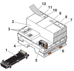
Fig. 5-3 Design of an XM21 controller
