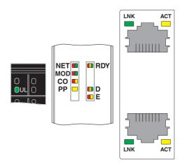
Fig. 9-1Indicators on bus couplers (example: S20-EIP-BK)All bus couplers in a F-BK housing have the following indicators:
