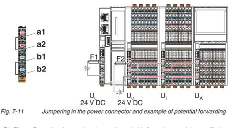
F1, F2 Protecting the supply voltage using suitable fuses (see module-specific documentation)
