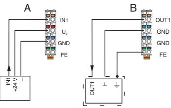
Fig. 7-17 3-wire connection for digital modules
