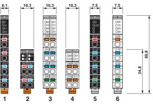
Fig. 5-19 Connectors: versions and dimensions
