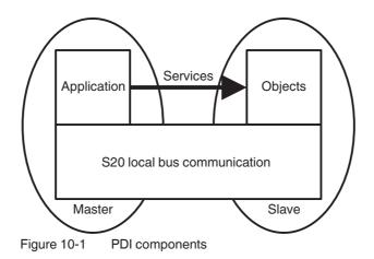
Every service access consists of a request and the associated confirmation. Only one service can be processed for an I/O module at a time.
