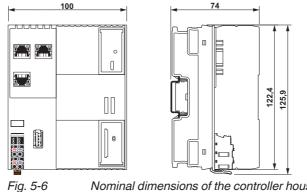
Nominal dimensions of the controller housing (type XM2x: e.g., XM21)
