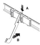
• Hook the shield bus holder onto the DIN rail.
