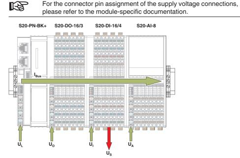
*Fig.* 7-10 Supply voltages in the IndraControl S20 system Key:
