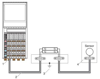
Fig. 8-10 Integration of analog shielding in a concept with central equipotential bonding at the control cabinet entry
