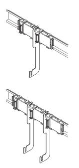
• Snap the shield bus holder onto the DIN rail.
