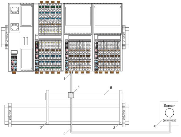
Fig. 8-9 Connecting the shielding to a busbar
