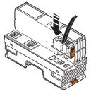
Fig. 7-7 Inserting the connector
