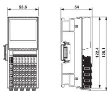
Fig. 5-10 Nominal dimensions of the F housing with one terminal field (type 1F: e.g., S20-AI-8, S20-DI-32/1)
